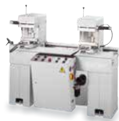
Pegaso 2 Electropneumatic drilling machine with two units and two spindles Electropneumatic drilling machine with two units and two spindles with automatic drill bit descent. The machine is equipped with two mobile heads with quick adjustment of the drilling axis along the Y axis by means of 8 preset mechanical stops.
