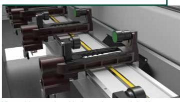
Vices with manual positioning and automatic locking of the longitudinal position are also available on request.
