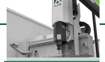
**MACHINING ON 5 PROFILE FACES** The machining head is compact in size to minimise the need for repositioning, but extremely rigid to guarantee excellent quality.
