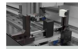
To extend the clamping capacity and the working areas, cast iron **EXTRA CLAM- PING VICES** are available, in which closing of the jaw is carried out using straight quides.
