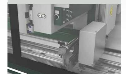
**MACHINING HEAD** allows machining operations to be carried out on 3 sides of the profile at any angle between 0° and 180° and on the 2 ends. The brushless motor allows exceptional performance in terms of acceleration and speed, placing the FMC 230 at the top of its category.
