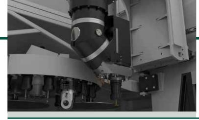
**ELECTROSPINDLE** Liquid cooled 24000 rpm, 22 kW HSK E63 electrospindle.
