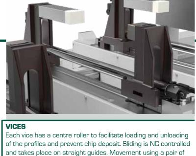
Gantry axes combats the high stress, generated by bending the bars, to which the vices are subjected during positioning. The vices can be configured quickly to adapt perfectly to the profile being locked, with wiring channels that are fully protected from chips and coolant fluids. Patented X RAISE vices with lifting support table are available on request.
