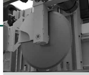
**X MODULE** this is the downfeed cutting unit driven by 4 controlled axes (x,y,z and rotation A) and Ø650mm blade. Two groups of motorised vices are provided for proper alignment and pneumatic locking of incoming and outgoing profiles. The vice surfaces are equipped with blowers to clean away any chips.
