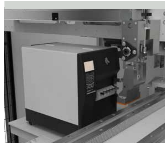
X LAB - AUTOMATIC PRINTER applying labels to the moving bar. The label can be applied to the top or rear side.
