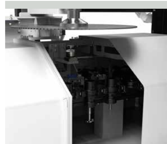
TOOL MAGAZINE automatic chain type with 32 locations plus the blade.
