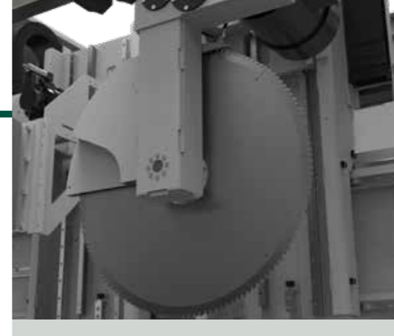
X MODULE is the downfeed cutting unit driven by 4 controlled axes (x,y,z and rotation A) and Ø 650mm blade. Two groups of motorised vices are provided for proper alignment and pneumatic locking of incoming and outgoing profiles.
