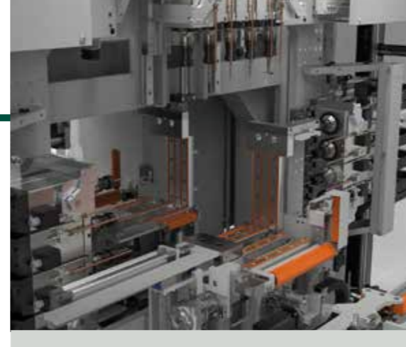
MULTI-SPINDLE MACHINING UNIT designed to carry out machining operations on all four sides of the profile. Tilting electrospindles are available with pneumatic or controlled drive rotation for oblique machining operations and electrospindles for rigid tapping. Designed to receive up to 18 HSK- C40 electrospindles.
