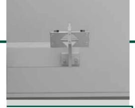
**X FLOW** dynamic orientation of lubrication nozzles (supplied as standard on FMC 370). **FOM INDUSTRIE PATENT**
