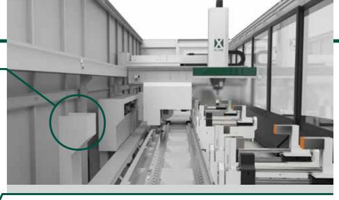
**X AXIS BEAM CARRIAGE** made of electrowelded steel. It moves on straight recirculating ball guides, with a brushless motor guaranteeing high performance. Working speeds of up to 100m/min.
