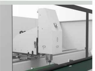
Made of electrowelded steel, it moves on high preci-Allows machining on 3 sides of the profile and on the 2 ends. On request, rotation of the work sion straight guides. Movement of the X, Y and Z axes table to intermediate angles with manual stop.
