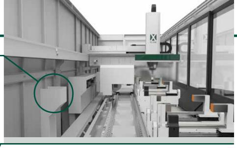
**X AXIS BEAM CARRIAGE** made of electrowelded steel. It moves on straight recirculating ball guides, with a brushless motor guaranteeing high performance. Working speeds of up to 100m/min.
